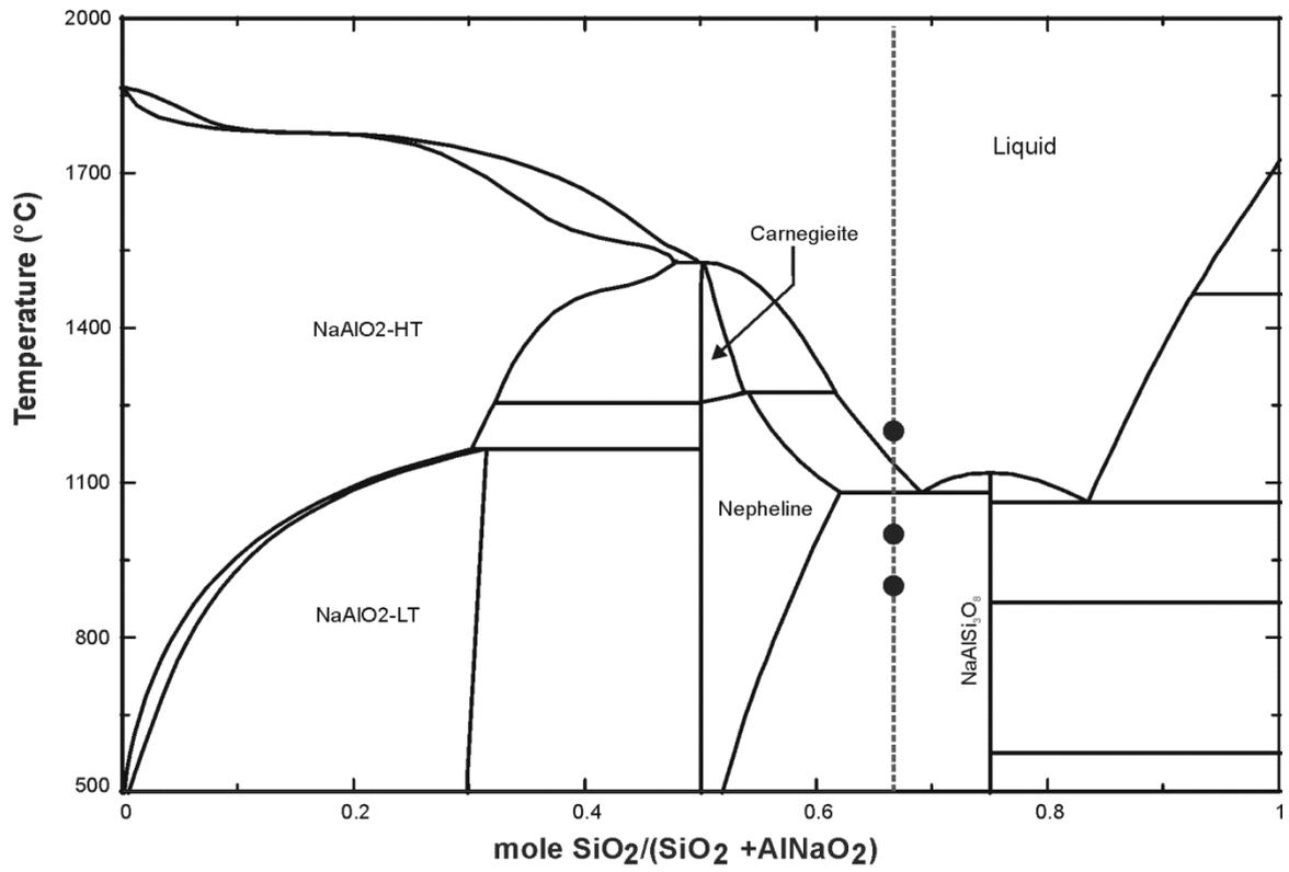
**Figure 10:** Phase diagram of NaAlO<sub>2</sub>-SiO<sub>2</sub> modeled using FactSage 6.3, the line represents the pure geopolymer mixture [38].
