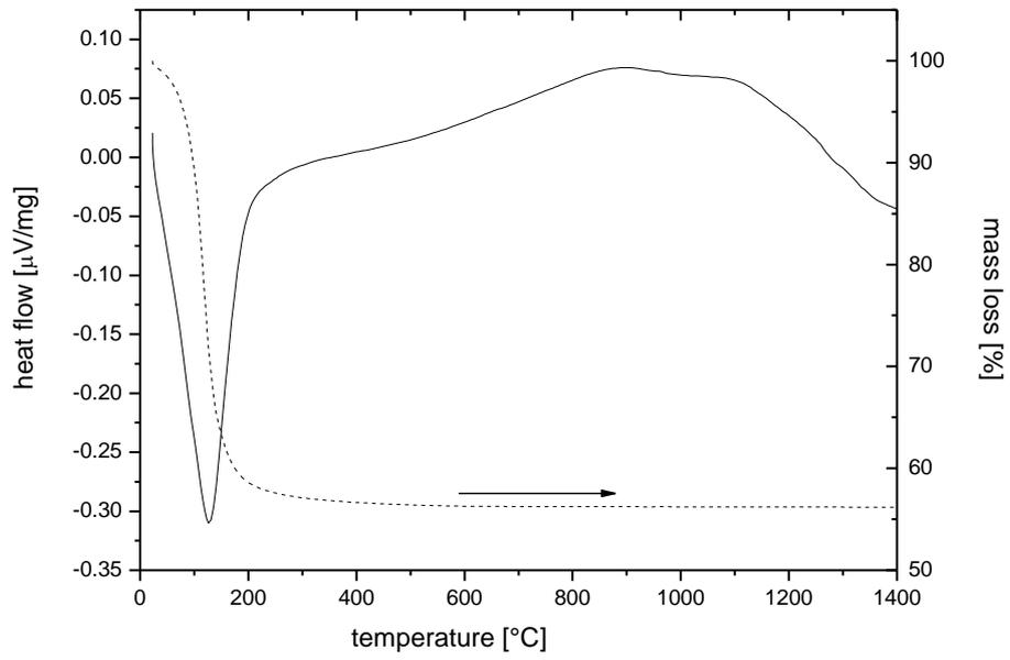
**Figure 2:** TGA/DSC data for 75 day cured metakaolin geopolymer (GP-pure) with Al:Si:Na:H<sub>2</sub>O molar ratio of 1:2:1:8.
