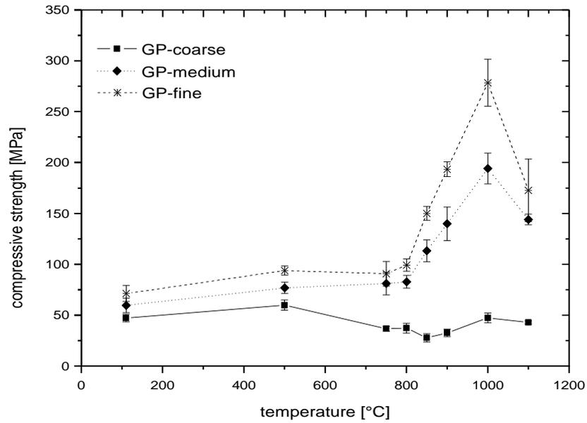
**Figure 4:** Compressive strength of geopolymer/sand mortar samples as a function of the heat treatment temperature. Data shown are the average and standard deviation of 5 measurements.
