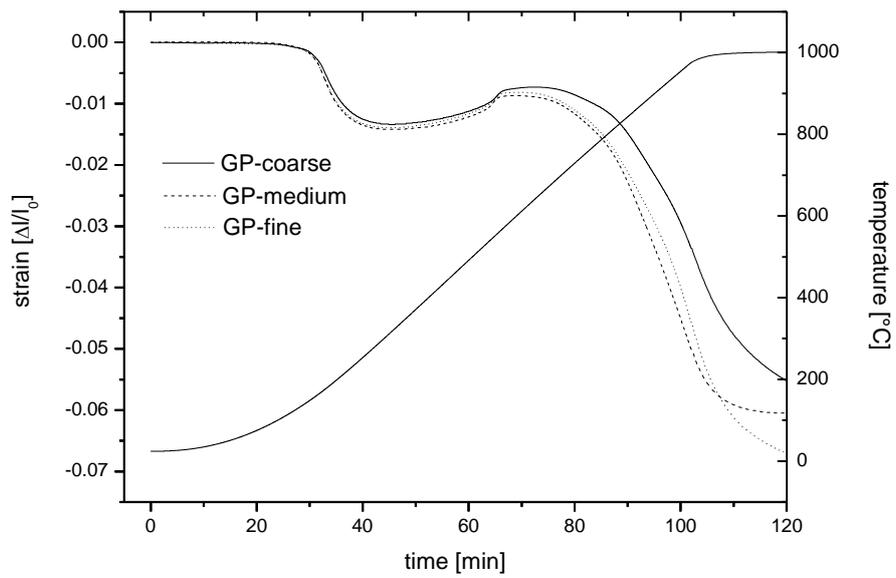
**Figure 3:** Dilatometer results the geopolymer mortar samples GP-coarse, GP-medium and GP-fine.
