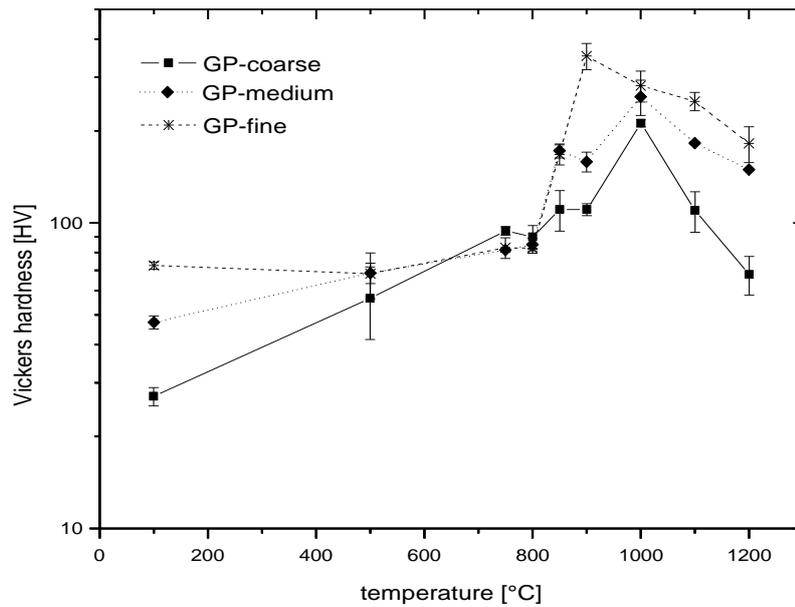
**Figure 6:** Change of hardness versus temperature for geopolymer samples (pure GP) containing no sand. Data points are averages of 9 measurements.
