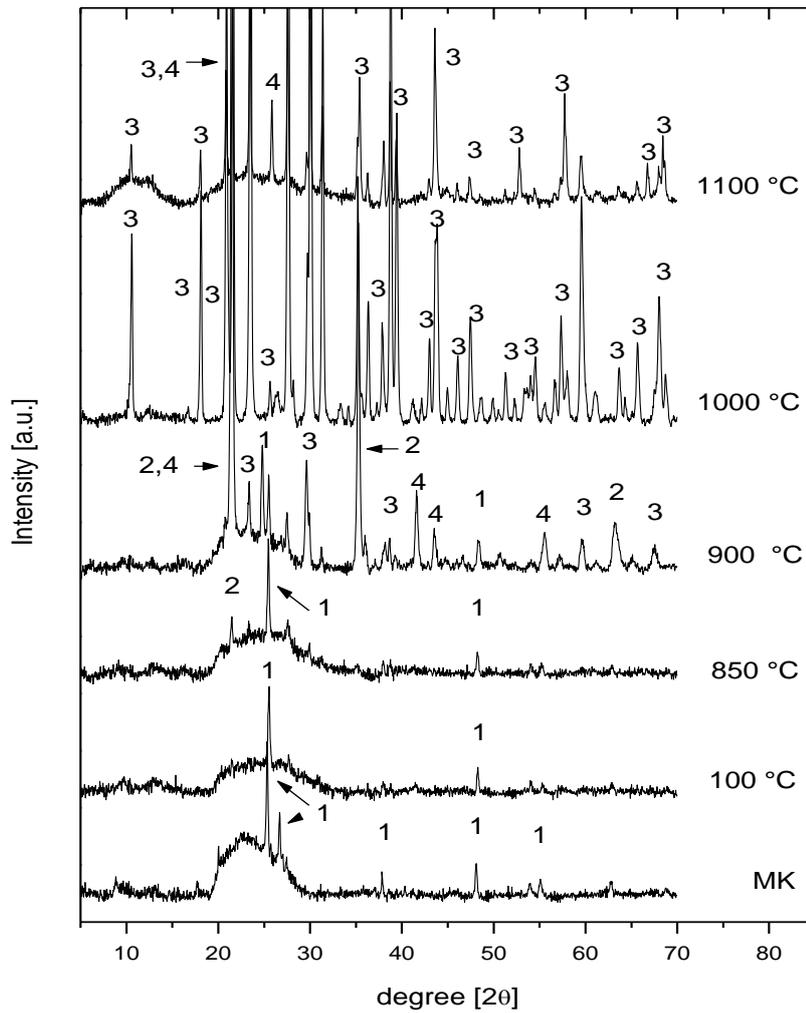
**Figure 8:** Change of crystalline phases after heating of pure geopolymer (pure GP) samples to different temperatures. Key: 1= quartz [ $\text{SiO}_2$ ], 2= sodium aluminium silicate [ $\text{NaAlSi}_2\text{O}_6$ ], 3= nepheline [ $\text{NaAlSiO}_4$ ], 4= carnegieite [ $\text{NaAlSiO}_4$ ].
