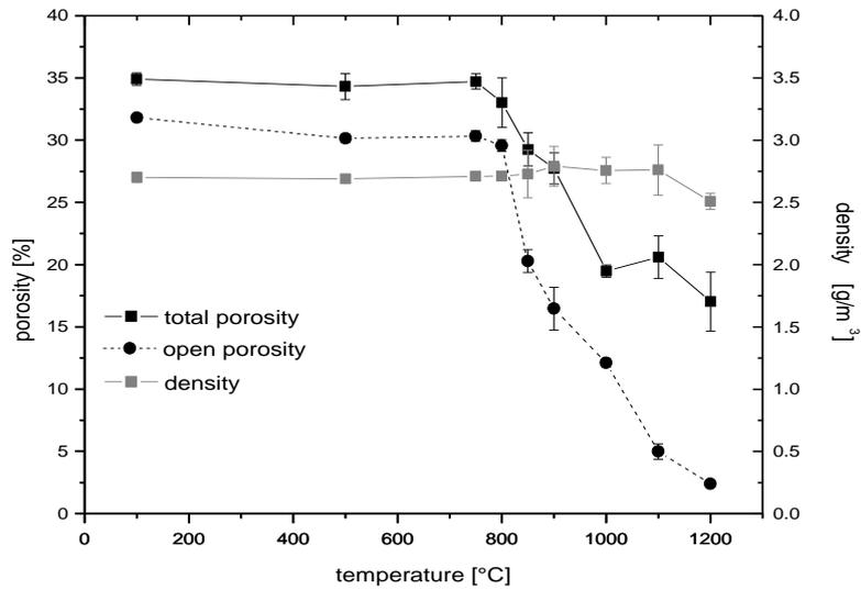
**Figure 7:** Porosity changes after exposure to different temperature for GP-medium. Very similar results were obtained for the other geopolymer mortar samples tested. Data presented is the average and standard deviation obtained from 5 measurements.
